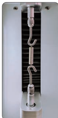
extension spring test
